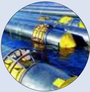
Pipes with end plugs, front cones and towing clamps ready for delivery (Montpellier, France, 2003)
