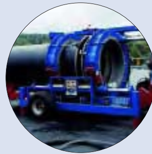
Welding of stubend on 1400 mm pipe (Reykavik, Iceland 2001)
