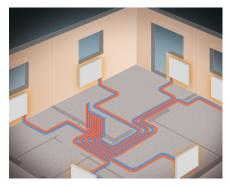
The heating manifolds are preassembled in the factory. The heating pipes are connected to the manifold by Eurocone connectors.
