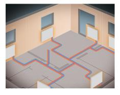
Do not perform the connection of heating bodies, manifolds and collectors directly in straight lines. To retain linear expansion, the pipes should be placed in the distance of approx. 1.5 m from a heating body, in the angle of 90°. This way the pipe system will absorb the linear expansion.
