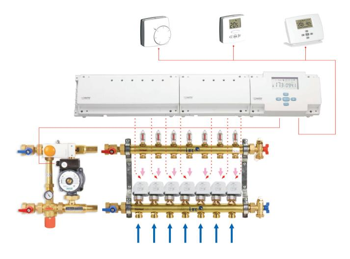
The room thermostats send signals for switching on and off to the Master junction box and the extender depending on the temperature. The junction box opens or closes the valve actuators and starts or stops the pump (also in the boiler) and the gas burner of the boiler if necessary. On the controller connected to the junction boxes, the switching on and off signals can be set (timed) for any period of the day and the week.
