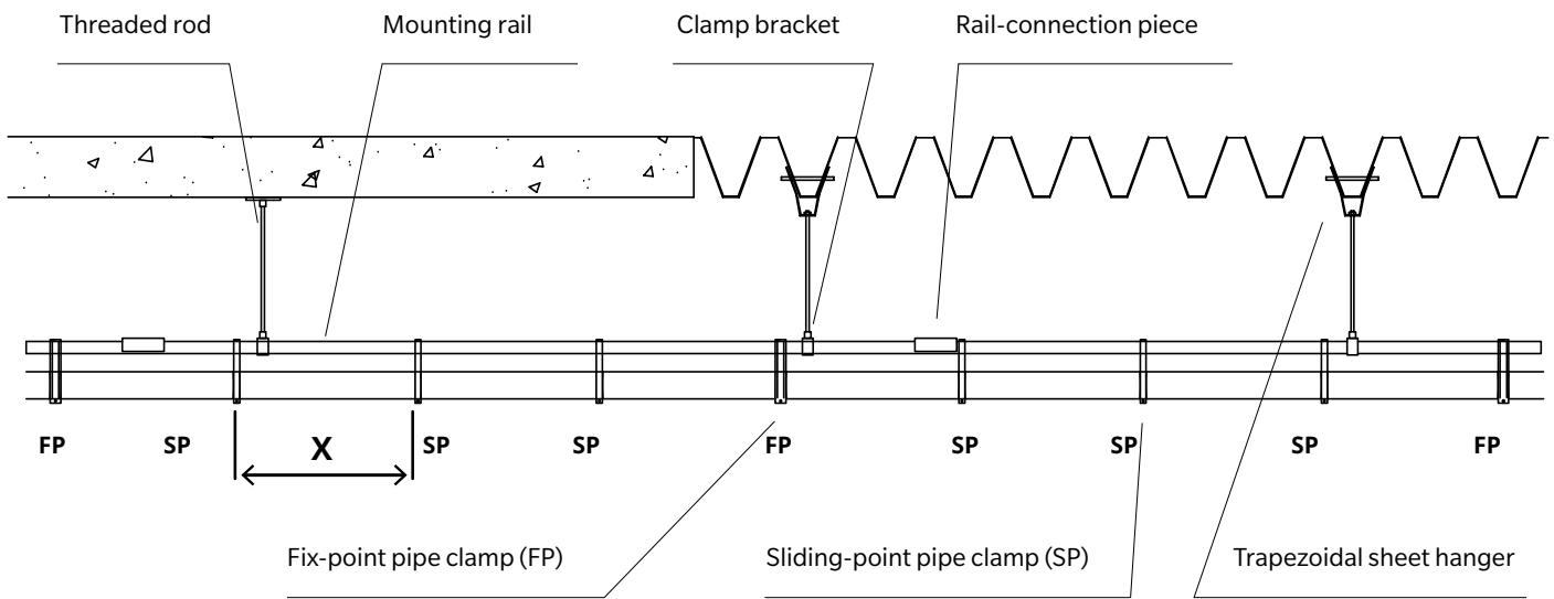
The minimum distance between mount points (X) depends on the diameter of the pipe.
