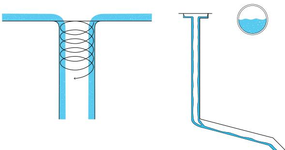
Conventional rainwater drainage systems utilize gravity to draw water into the downpipes. However, this also allows air to enter, causing the water to vortex along the pipes walls and reduce drainage flow rates.
