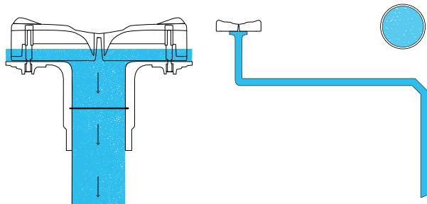
Siphonic outlets utilize air baffles to prevent air from entering the pipeline and inhibit the formation of the vortex.
