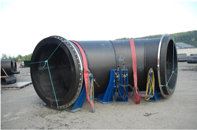
Fabricated 90 deg bend fitting for OD2000 mm
