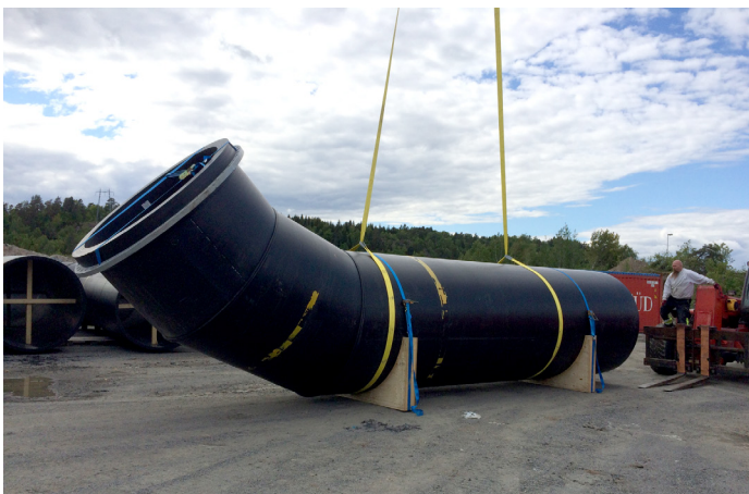
OD2100 mm SDR26 incorporated bend
